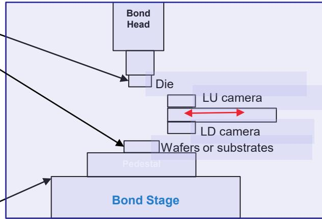
bonding tool schematic
