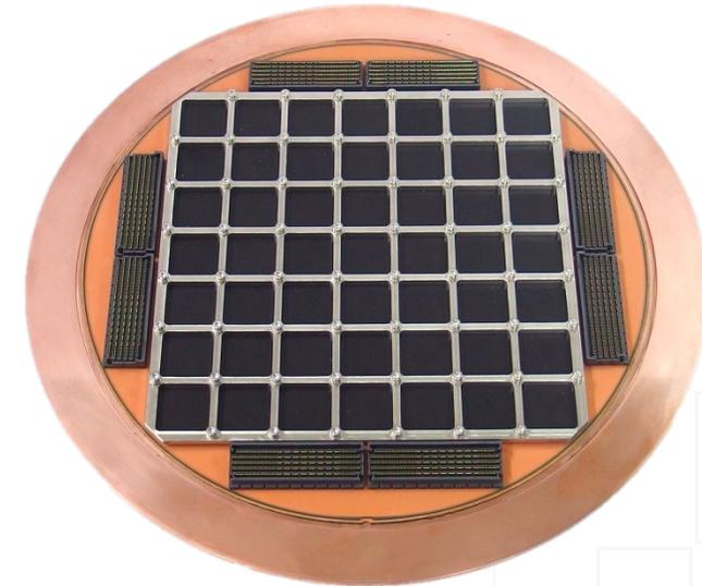
This SoW design posts significant challenges from defect inspection point of views from the algorithms and memory point of view comparing to other packaging.
