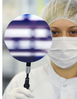
Osram 6" LED Epiwafer
